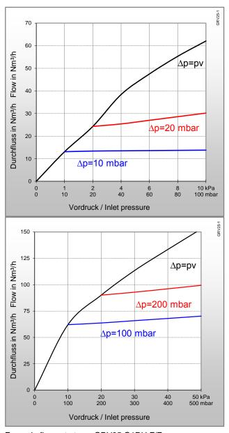
Example flow rate type: GRV25 G1RH F/F. Values for other connections on request.
